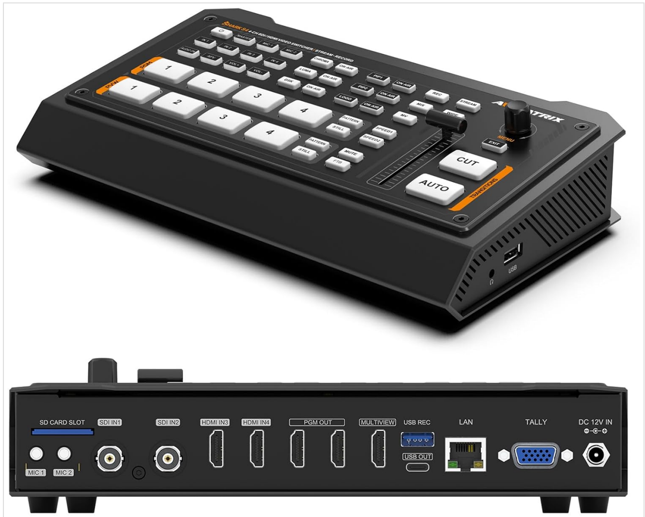
Figure 4.1: Top and Rear View of the AVMATRIX SHARK S4. The top view displays the control surface with input selection buttons, T-bar, and effect controls. The rear view shows all connectivity ports.
