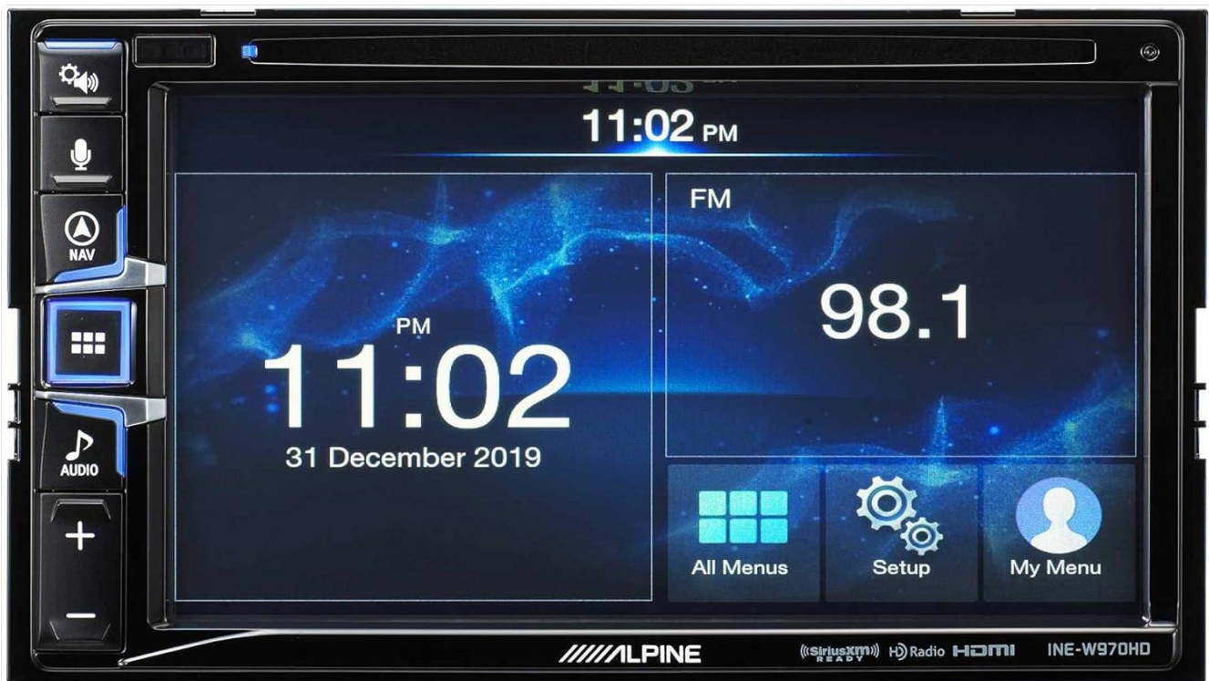
Image: The Alpine INE-W970HD head unit displaying the radio interface, showing frequency and time information.
