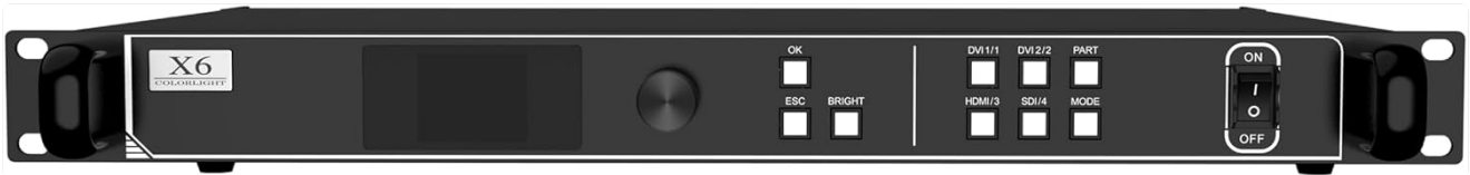
Figure 5.1: Front panel controls of the Colorlight X6.
