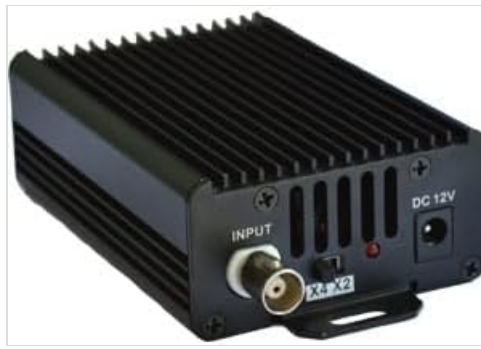
Figure 3.2: Side view of the amplifier, highlighting the integrated heatsink fins for efficient thermal management.
