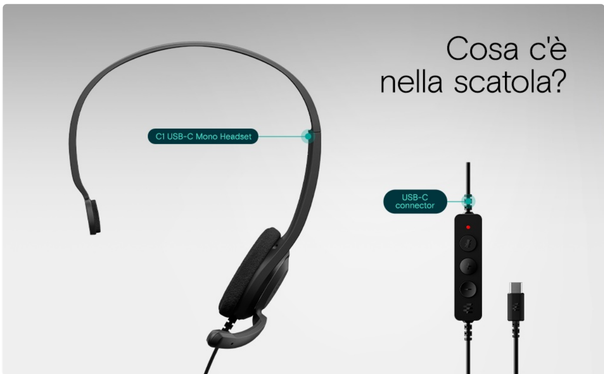
Figure 1: Package Contents. The image displays the EPOS C1 USB-C Mono Headset and its integrated USB-C cable with in-line controls, illustrating what is included in the product box.
