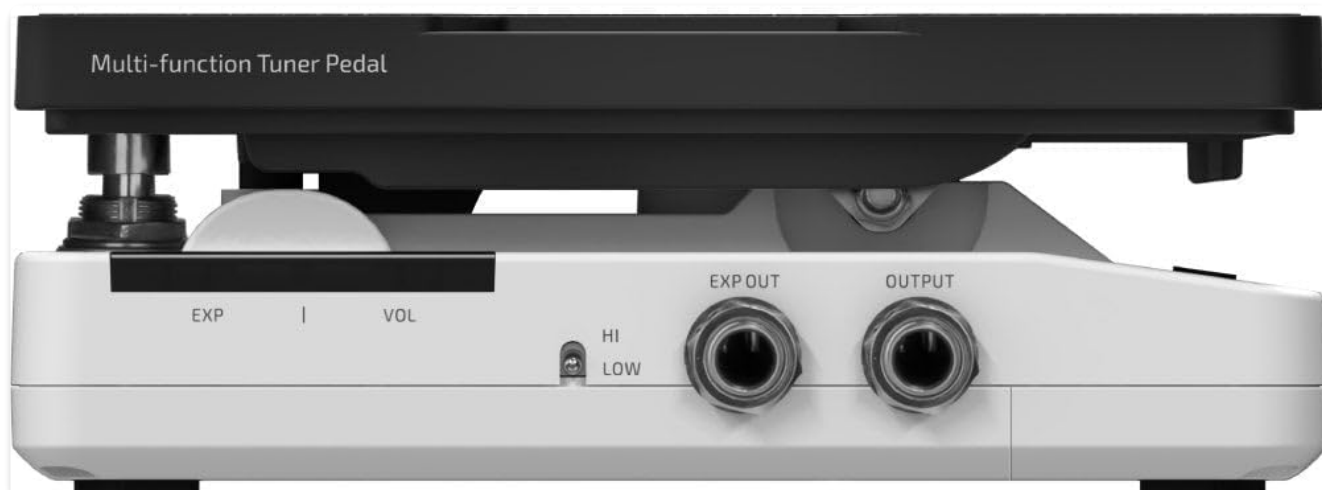
Side view of the pedal with output and expression connections, including the HI/LOW impedance switch.
