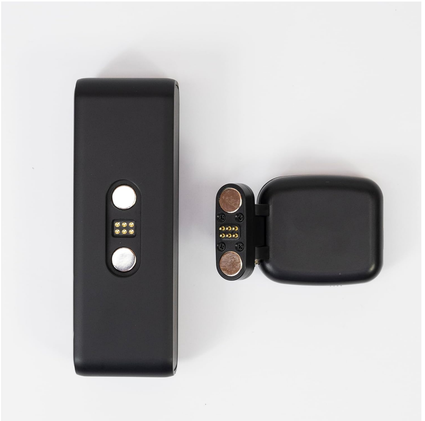
Image 5.1: The PNI Voyager S2600 dash cam detached from its magnetic mount, illustrating the contact points for secure attachment.
