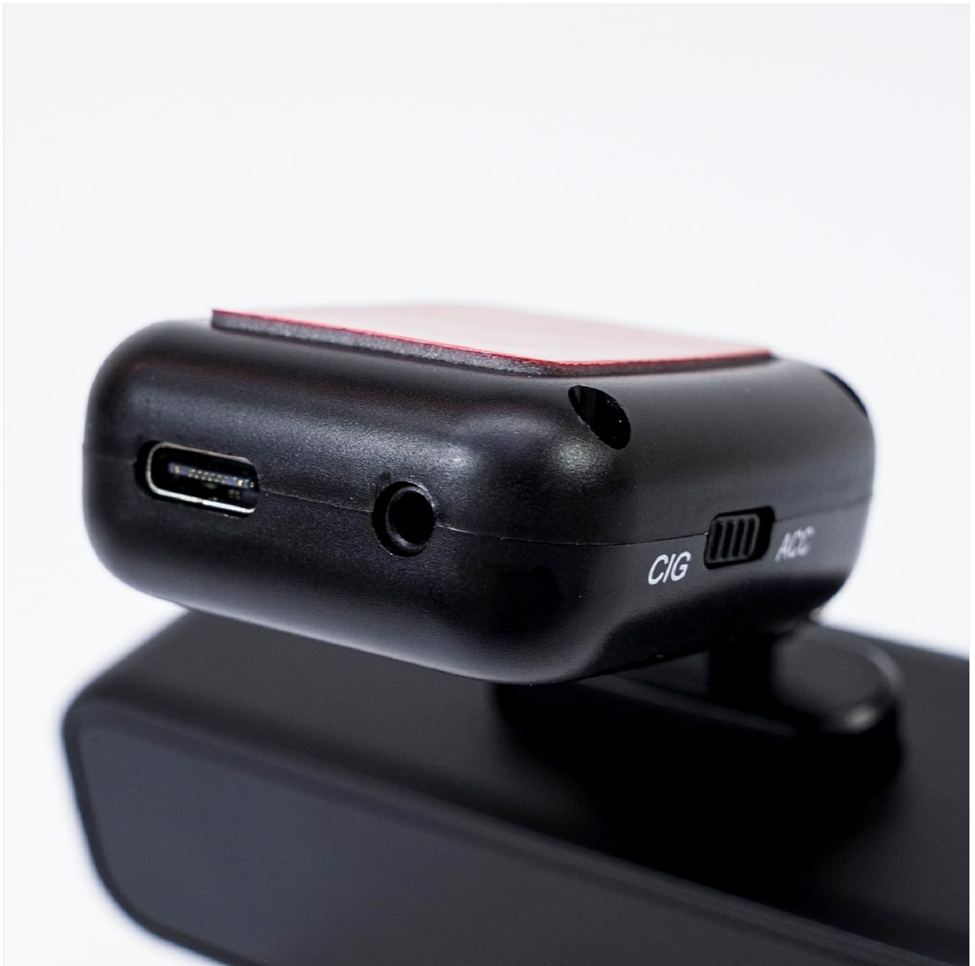
Image 5.2: The top of the dash cam mount, featuring the USB-C port for power input and the CIG/ACC switch for power mode selection.
