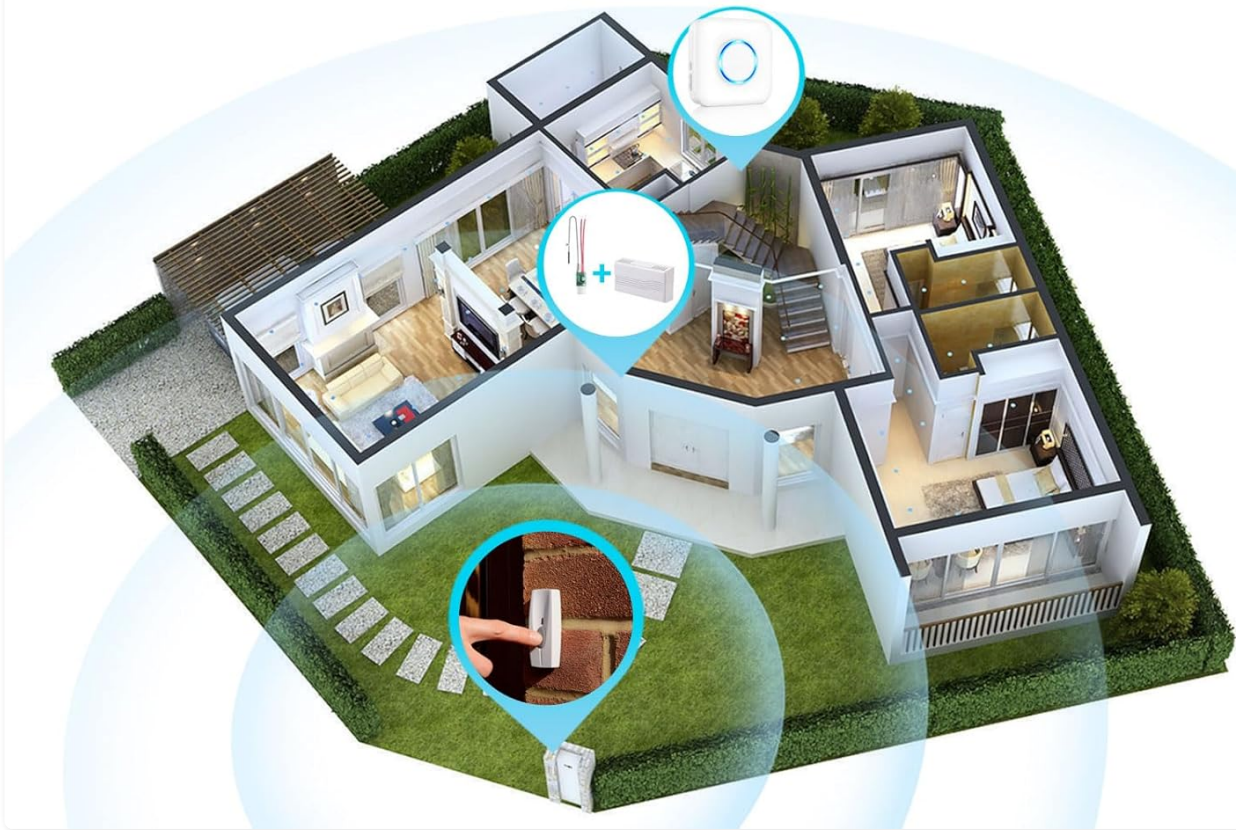
Image 1.2: This diagram illustrates the extensive coverage of the doorbell extender, reaching up to 656 feet (200 meters) in open areas, ensuring reliable signal transmission throughout a home or business, even through different types of doors.
