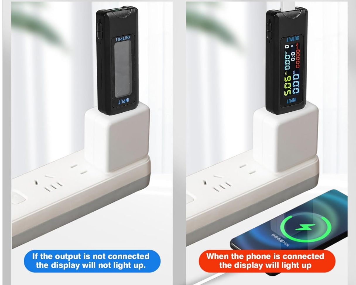
Figure 4: Illustration showing that the display will not light up if the output is not connected to a device, but will illuminate when a phone is connected for charging.
