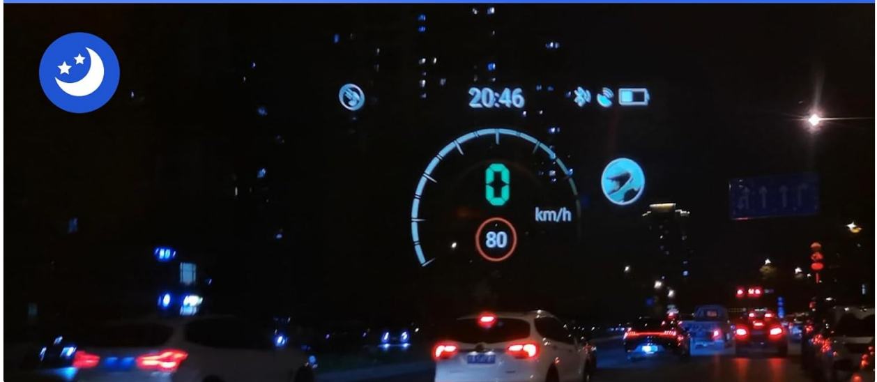
Image illustrating the automatic brightness feature of the HUD, showing clear display visibility during both day and night riding conditions.
