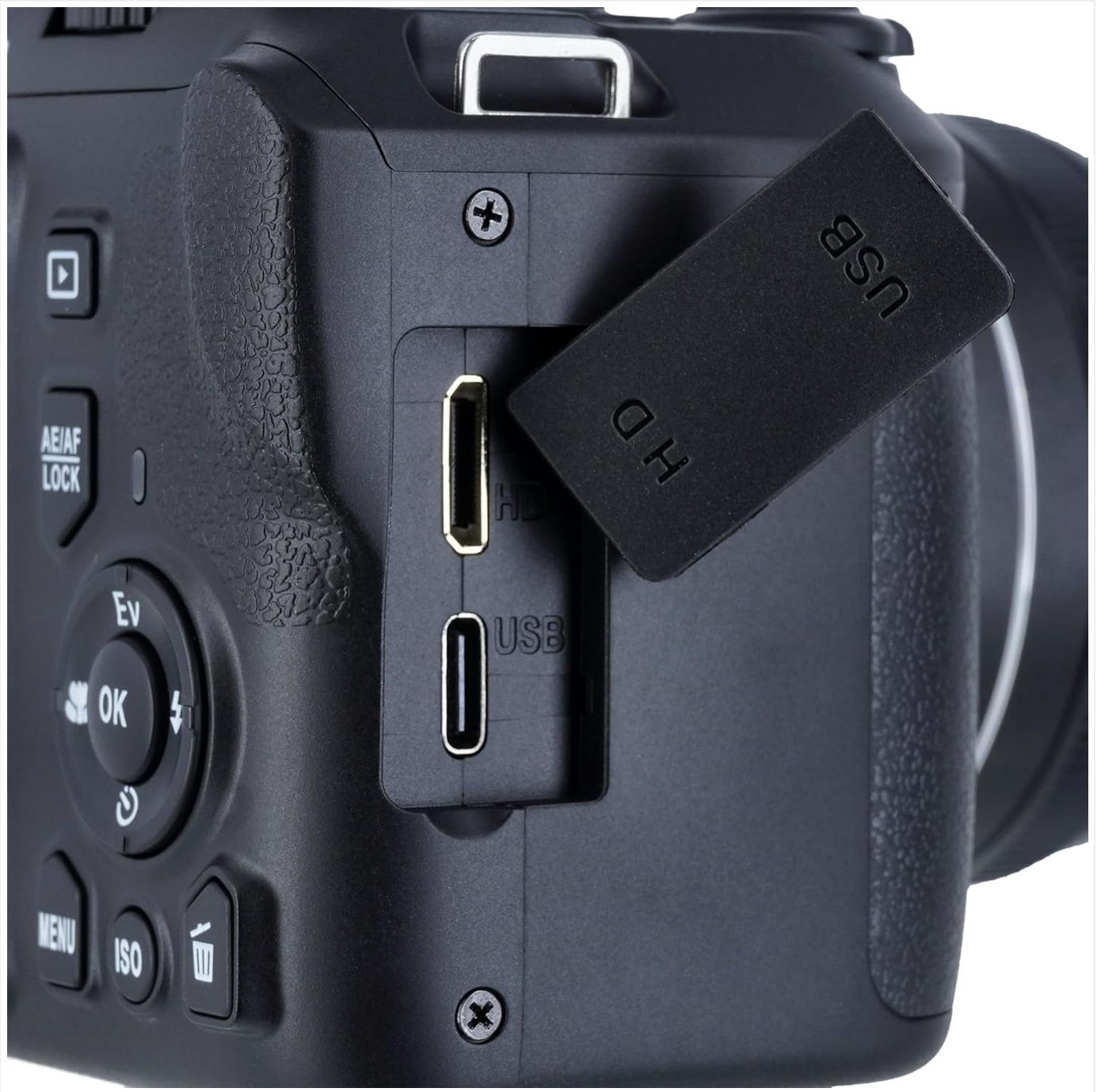
Figure 3: Side view of the camera with the protective cover open, revealing the USB and HD (HDMI) ports for connectivity.
