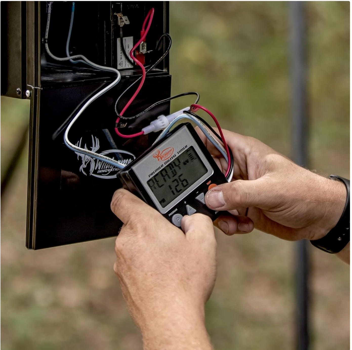
Figure 4: A user adjusting the settings on the digital timer, which controls the feed times and duration.
