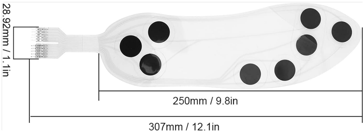
Figure 3: Approximate dimensions of the Topyond ZNX-01 detection mat.
