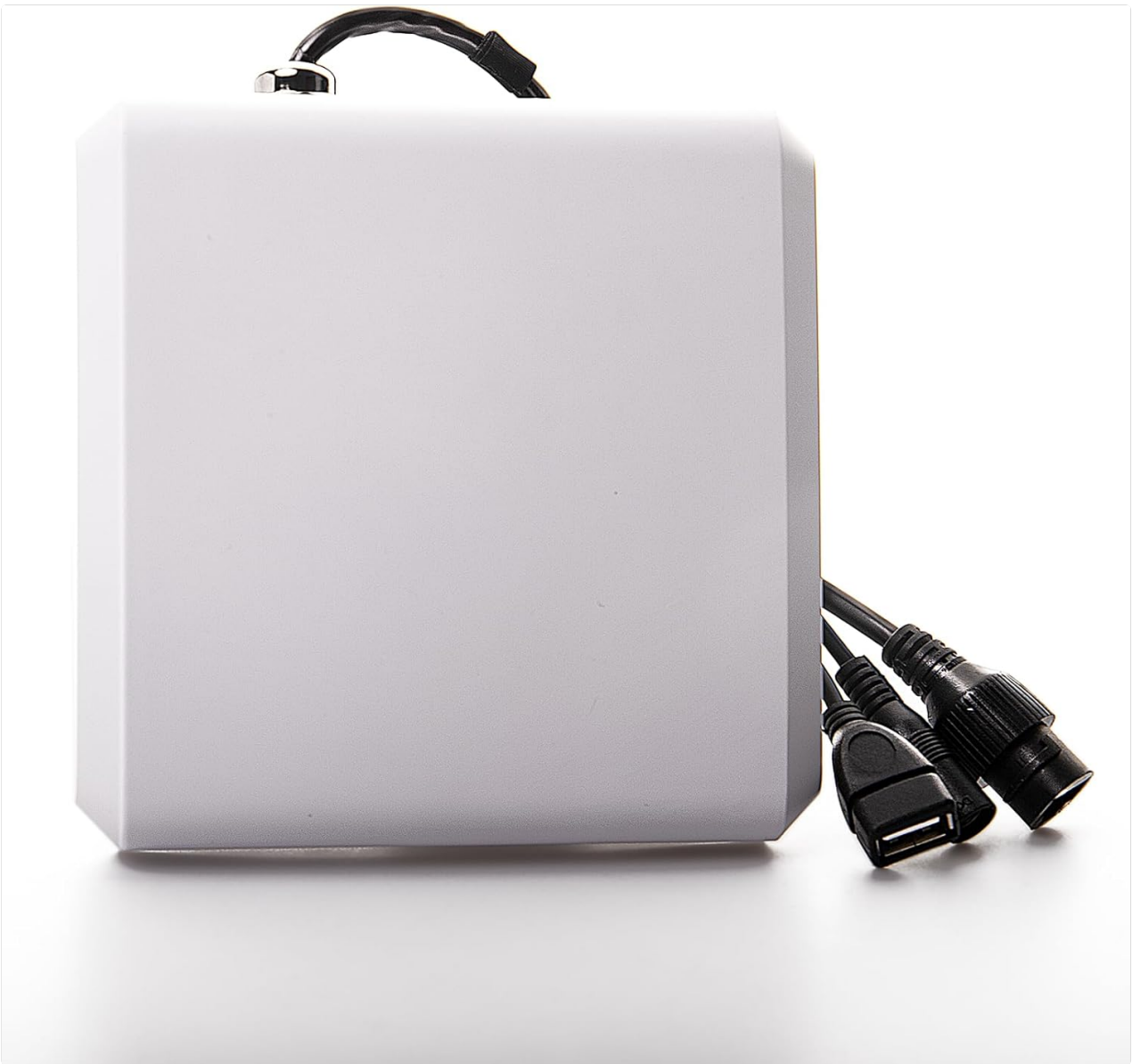
Figure 4.1: Front view of the Fongwah U6 RFID Reader with its connected USB and power cables.
