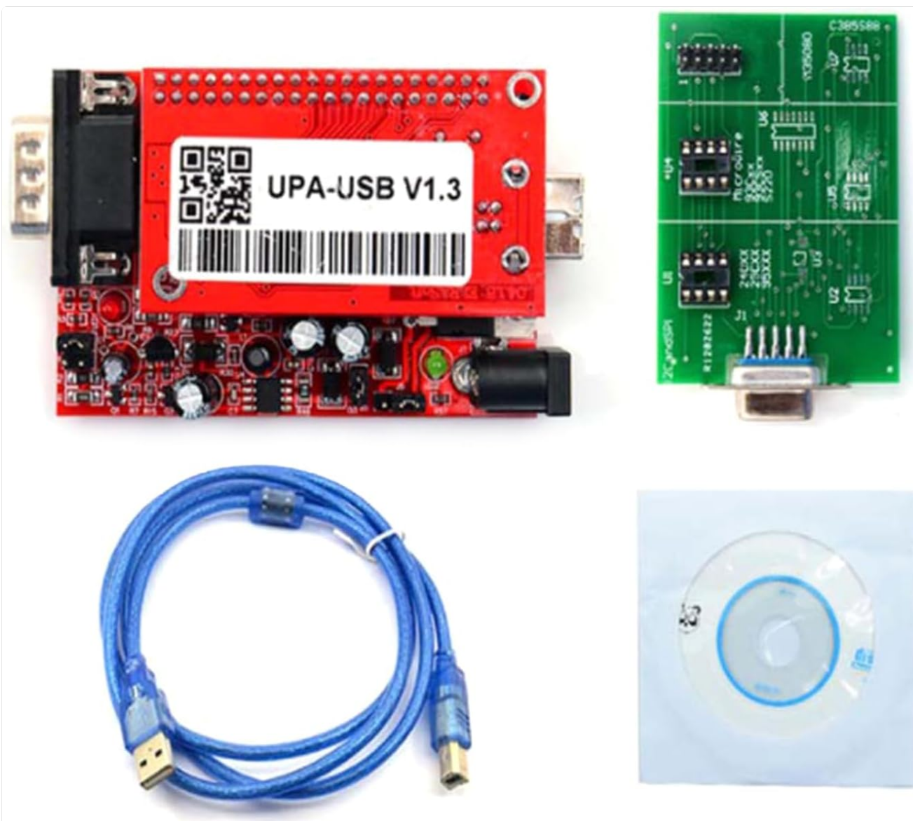
Figure 3.1: Main components of the Automotive Programming Tool, including the UPA-USB V1.3 main unit, a green adapter board, a blue USB cable, and a software CD.
