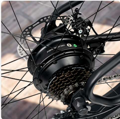
View of the rear wheel's hub motor and disc brake system.
