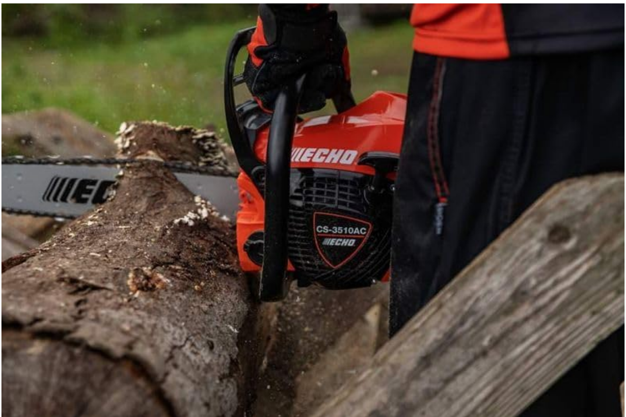
Figure 5.3: A close-up view of the chainsaw's chain engaging with a log during operation.
