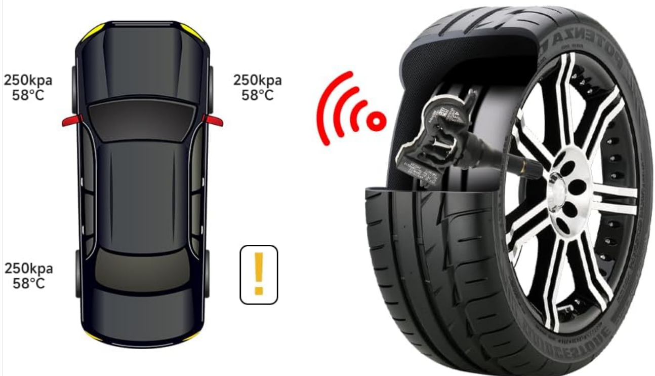
Figure 4: Visual representation of TPMS sensor alerts for various tire conditions.
