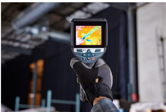
Figure 5.2: Thermal inspection of ductwork to identify temperature anomalies.
