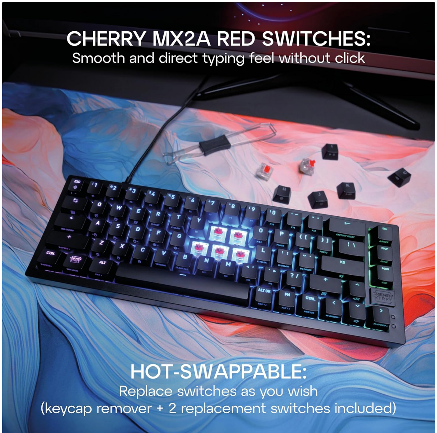
Figure 3: Detail of the hot-swappable Cherry MX2A RED switches, emphasizing their smooth, direct feel and ease of replacement.
