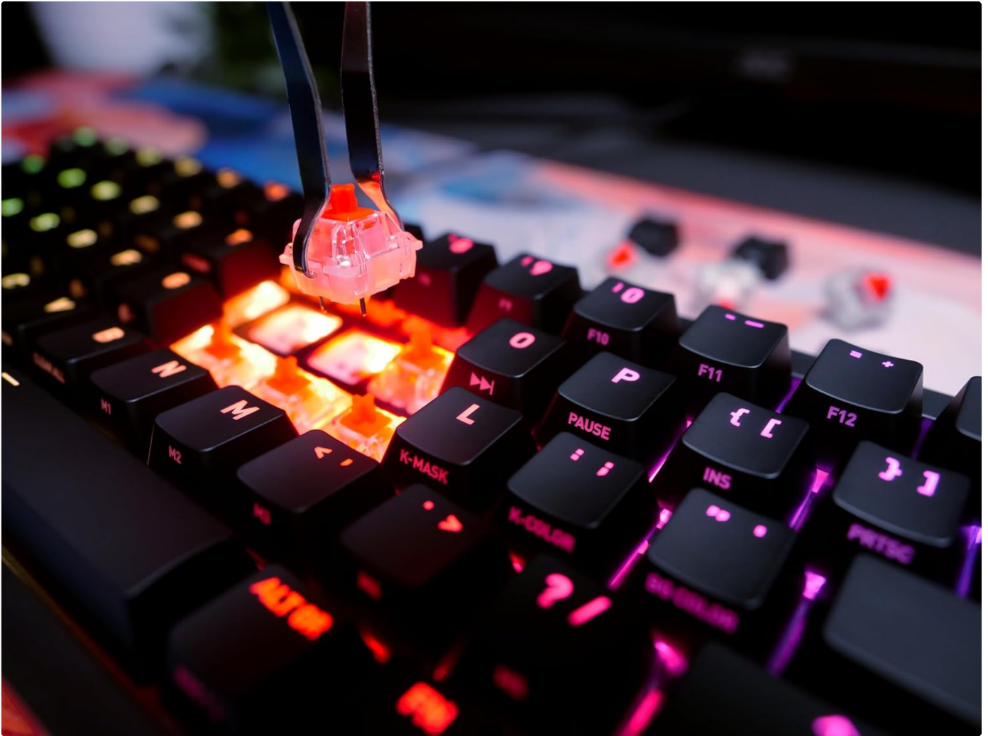
Figure 5: Demonstrating the process of removing a switch from the keyboard for replacement or customization.
