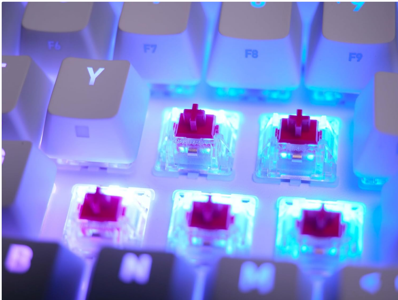
Figure 6: A detailed view of the Cherry MX2A RED switches, highlighting their design and the integrated RGB lighting.
