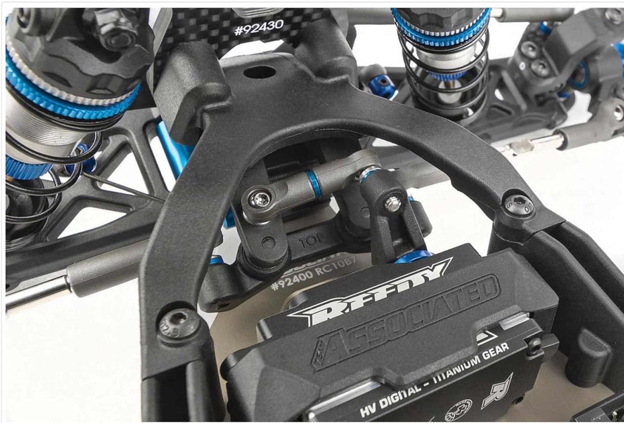
Figure 3: Detail of the 5-gear laydown transmission and the low-profile motor mount, centralizing weight for enhanced performance.
