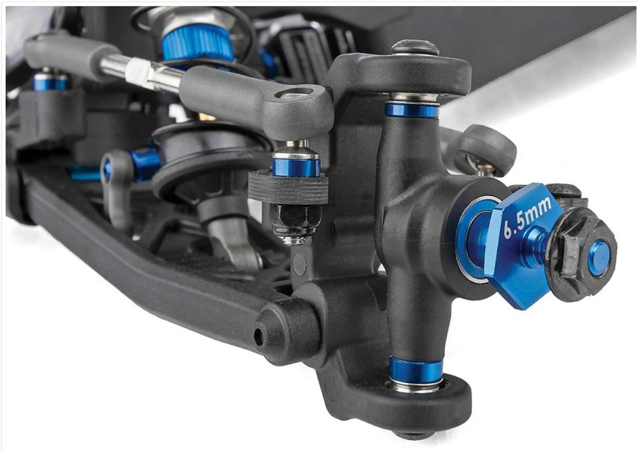
Figure 2: Close-up view of the front suspension, showing the KPI adjustable steering block and associated linkages, crucial for fine-tuning steering response.
