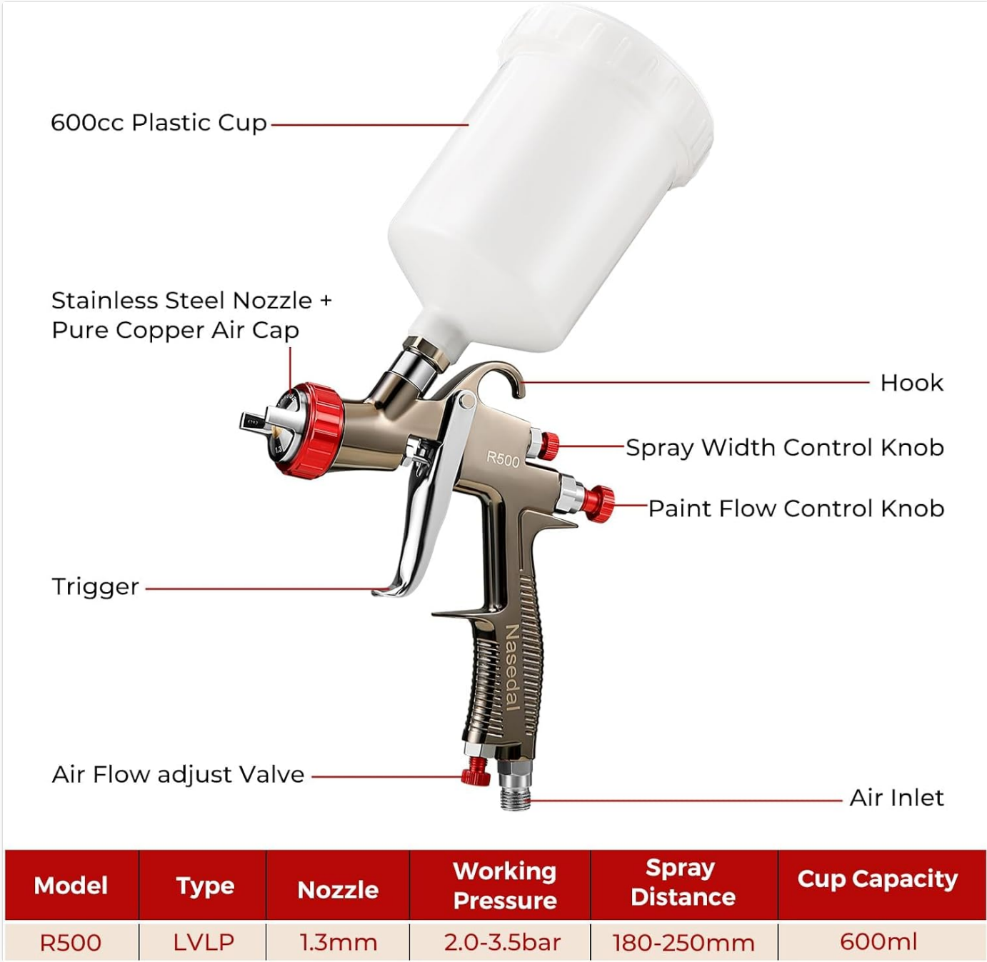
Image: Key components of the R500 spray gun, including the paint cup, nozzle, control knobs for spray width, paint flow, and air flow, trigger, and air inlet.
