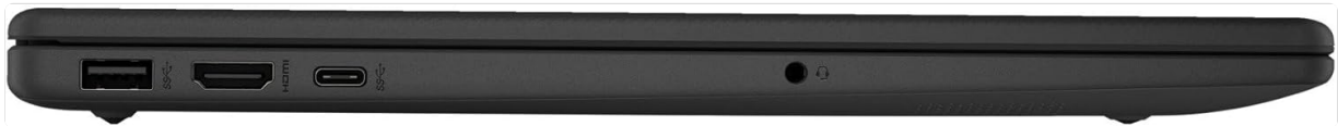
Figure 3.2: Left side ports including USB Type-A, HDMI, USB Type-C, and headphone/microphone combo jack.
