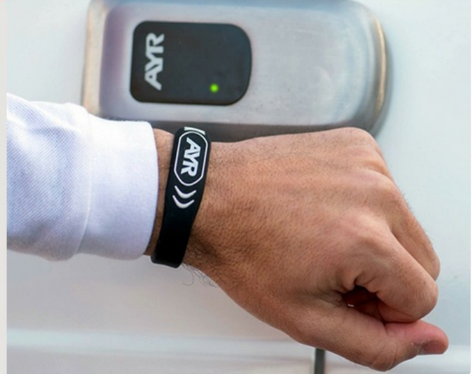
Image 4.1: Demonstrating the use of the NFC bracelet for quick access.
