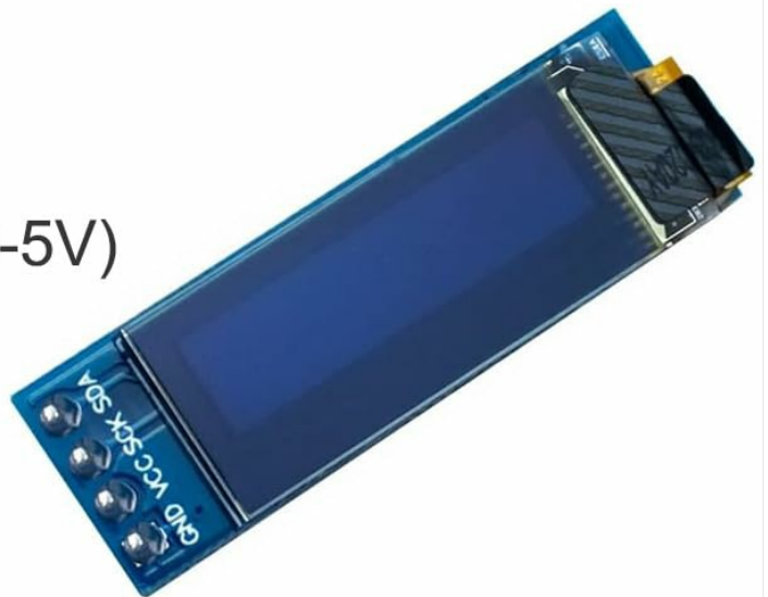
Image 4.1: Pinout diagram for the 0.91 inch OLED module, showing GND, VCC, SCL, and SDA connections. The module features a 4-pin interface for I2C communication. The pins are defined as follows:
