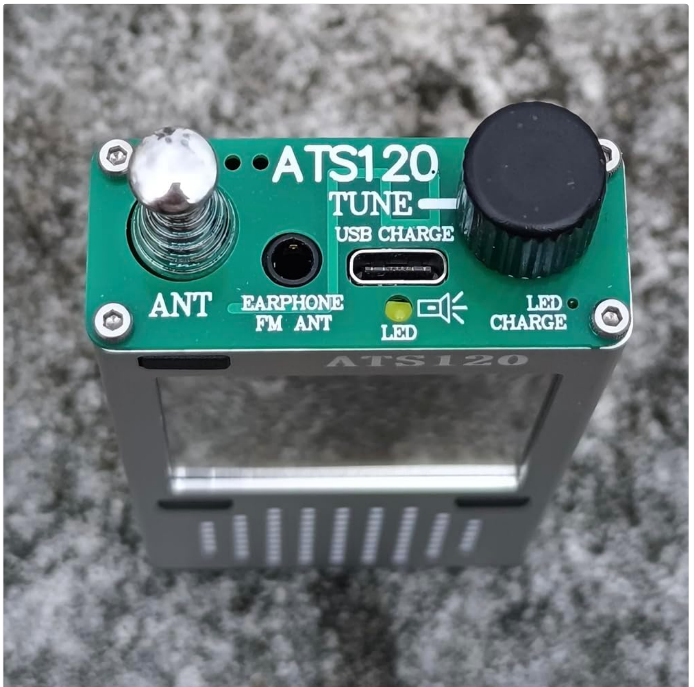
Figure 3: Top panel of the ATS120, featuring the retractable antenna, 3.5mm earphone jack (also functions as FM antenna input), USB-C charging port, and the main rotary encoder knob for tuning.
