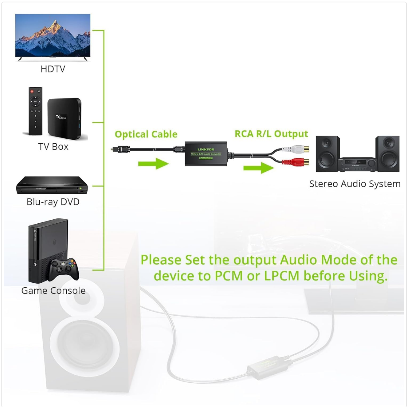
Figure 4.1: Connection Diagram. This diagram illustrates how to connect various digital audio sources (HDTV, TV Box, Blu-ray DVD, Game Console) to the LiNKFOR DAC Converter via an optical cable, and then connect the converter to a stereo audio system using RCA L/R outputs. A reminder to set the audio output mode to PCM or LPCM is included.
