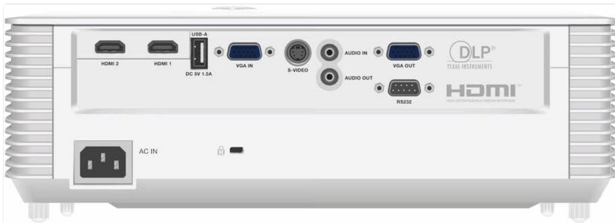
Figure 4.3: Rear view displaying the various input and output ports, including HDMI, USB-A, VGA, S-Video, Audio In/Out, and RS232.
