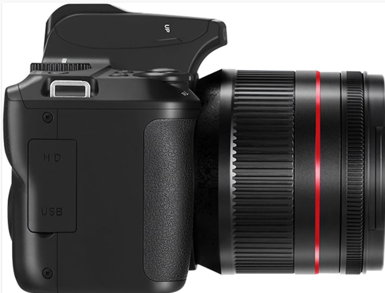
Figure 3.4: Left side view of the Ordor G700 Digital Camera, indicating the microphone input port.
