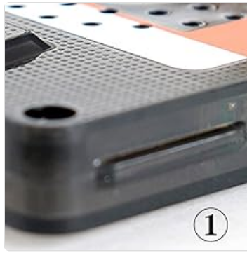
Figure 4.2: The microSD card slot, located on the side of the speaker, for direct audio playback.
