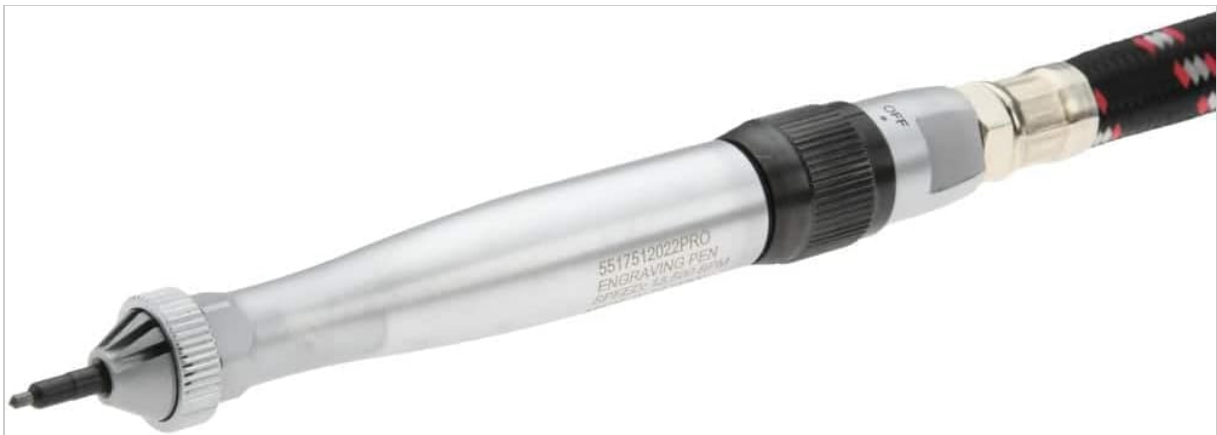
Figure 2.2: Close-up view of the engraving pen, detailing the throttle control and the model number (5517512022PRO) inscribed on the body.
