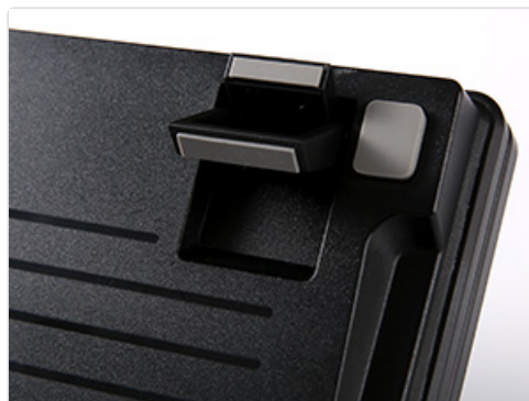
Figure 5: Mac/Win and connectivity mode switches.
