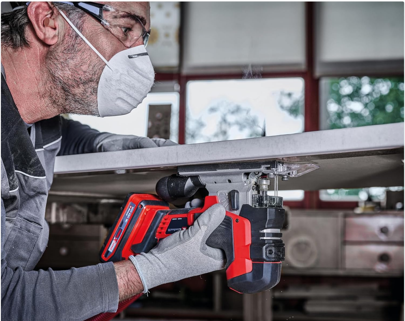
Image 5.1: A person wearing safety glasses and a mask, operating the Einhell jigsaw to cut a workpiece from below, demonstrating the tool's versatility in different working positions.
