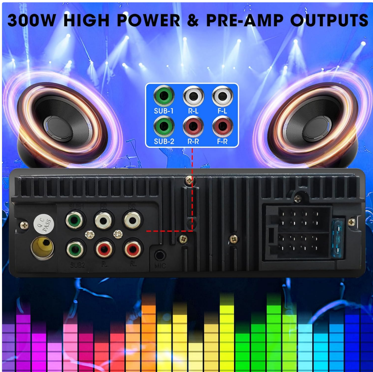
Figure 4.2: Rear Panel with RCA Outputs. This image displays the rear of the car radio, showing the various ports including RCA outputs for subwoofer (SUB-1, SUB-2), rear left (R-L), rear right (R-R), front left (F-L), and front right (F-R) channels, indicating its 300W high power and pre-amp capabilities.
