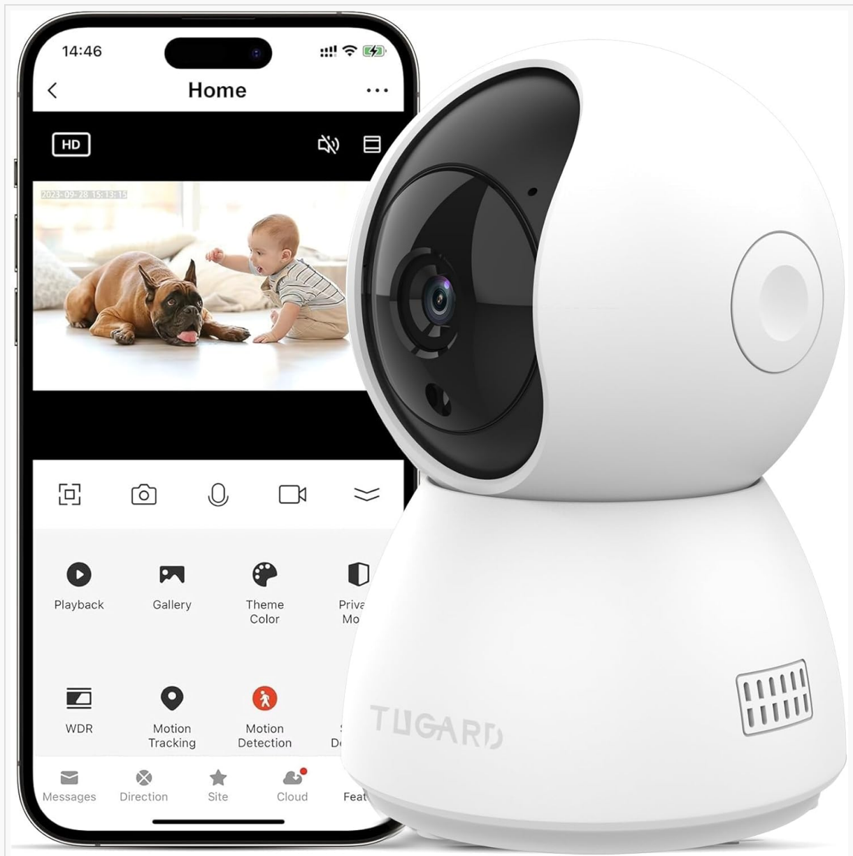
Image: The TUGARD ZASD-C23 camera positioned next to a smartphone showing the live view and control options within the Smart Life application.
