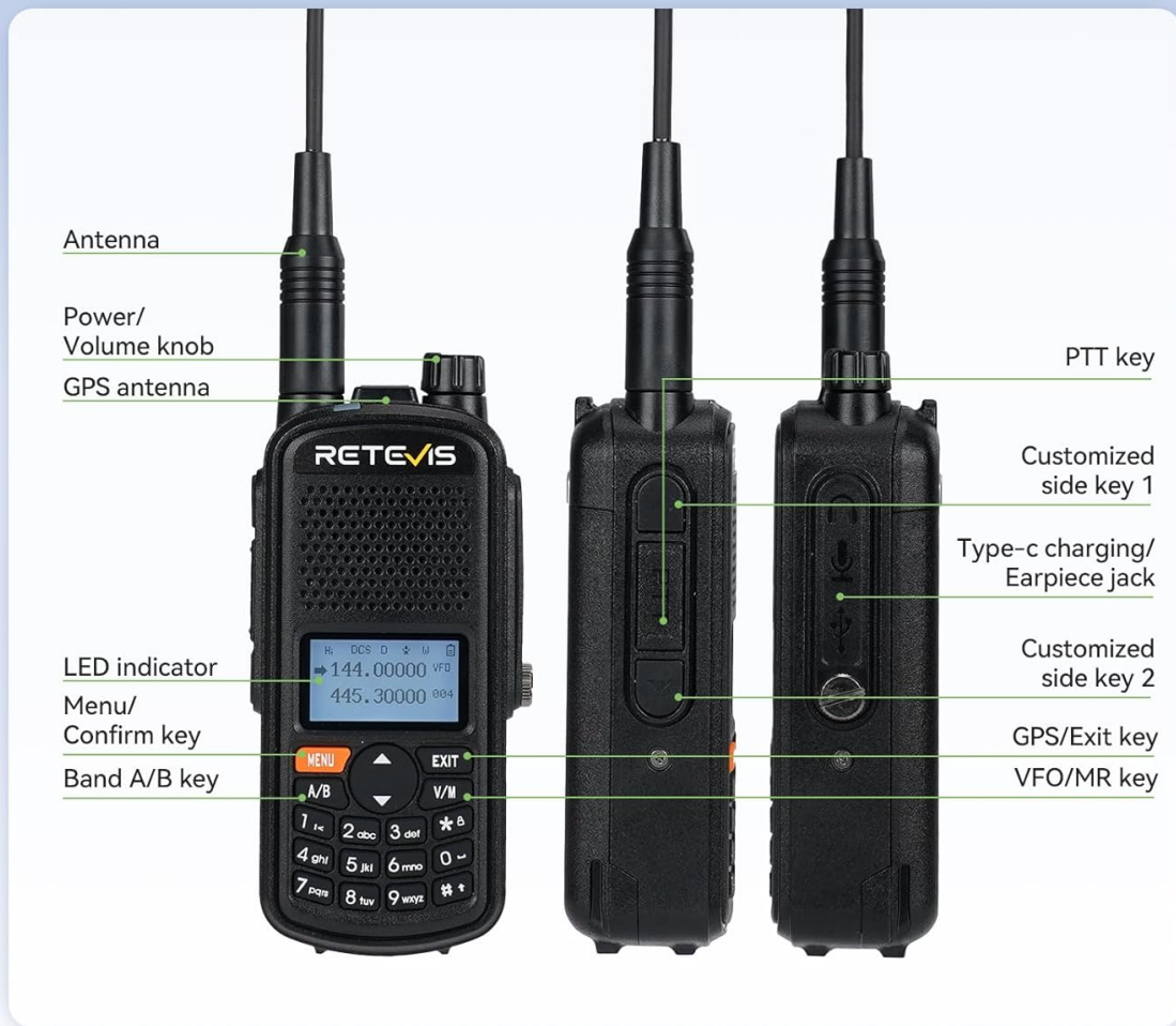
Figure 2: Detailed view of the Retevis A61 radio showing antenna, power/volume knob, GPS antenna, PTT key, customized side keys, USB-C charging port, earpiece jack, LED indicator, Menu/Confirm key, and Band A/B key.
