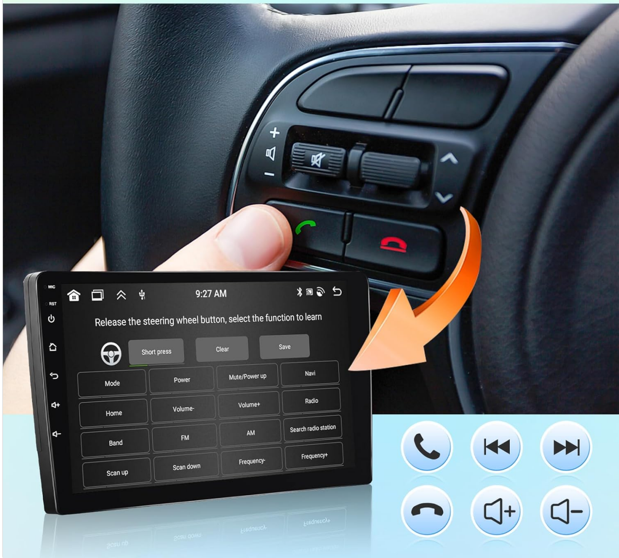
Image: The car stereo display showing the Steering Wheel Control learning interface, with an inset image of a steering wheel highlighting the control buttons.
