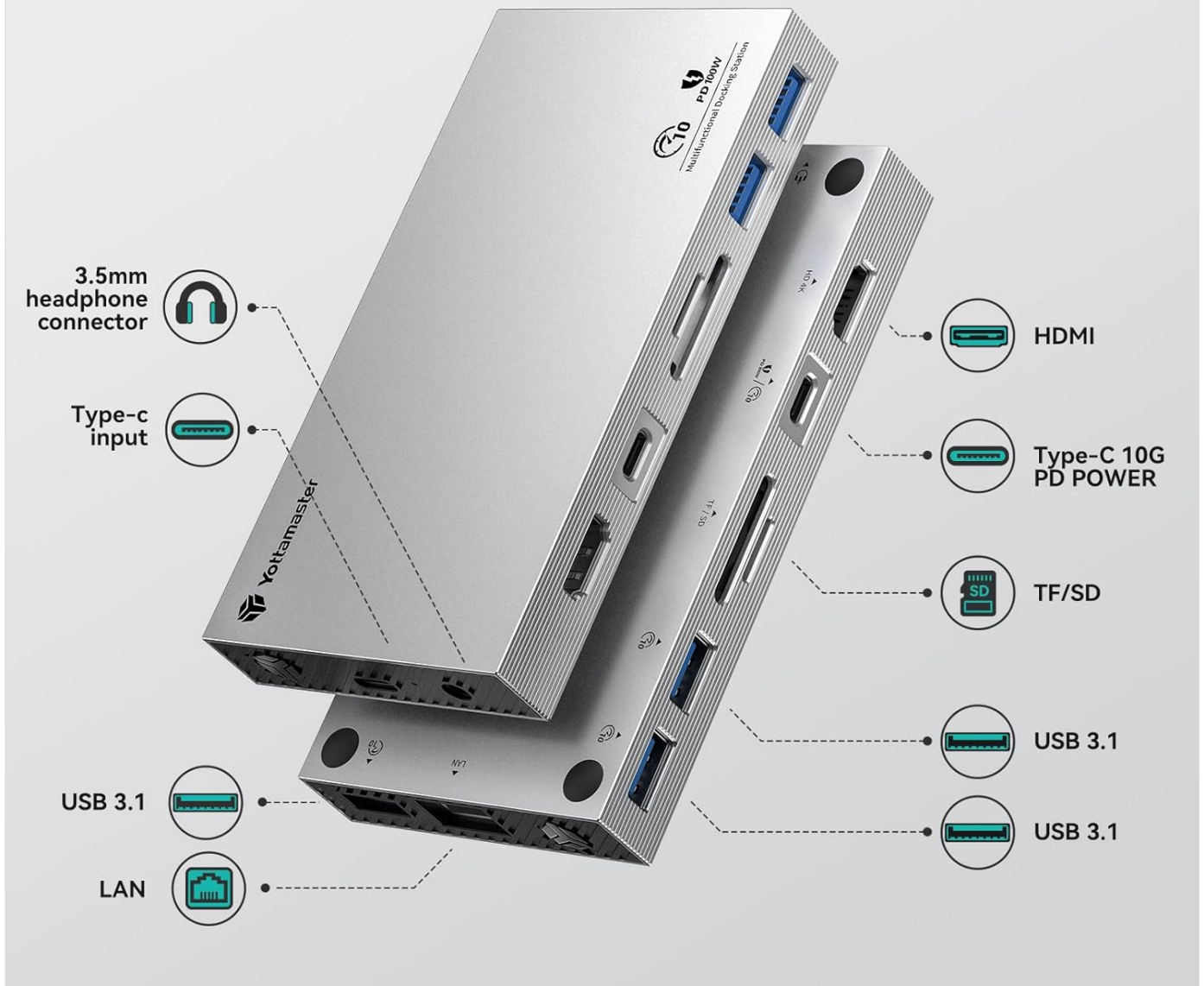
Image: A detailed diagram highlighting each of the 10 ports on the Yottamaster DS03CS and their respective functions.
