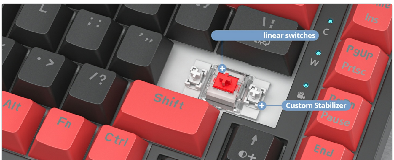
Image 5.6: Close-up view of linear switches and the custom stabilizer mechanism.
