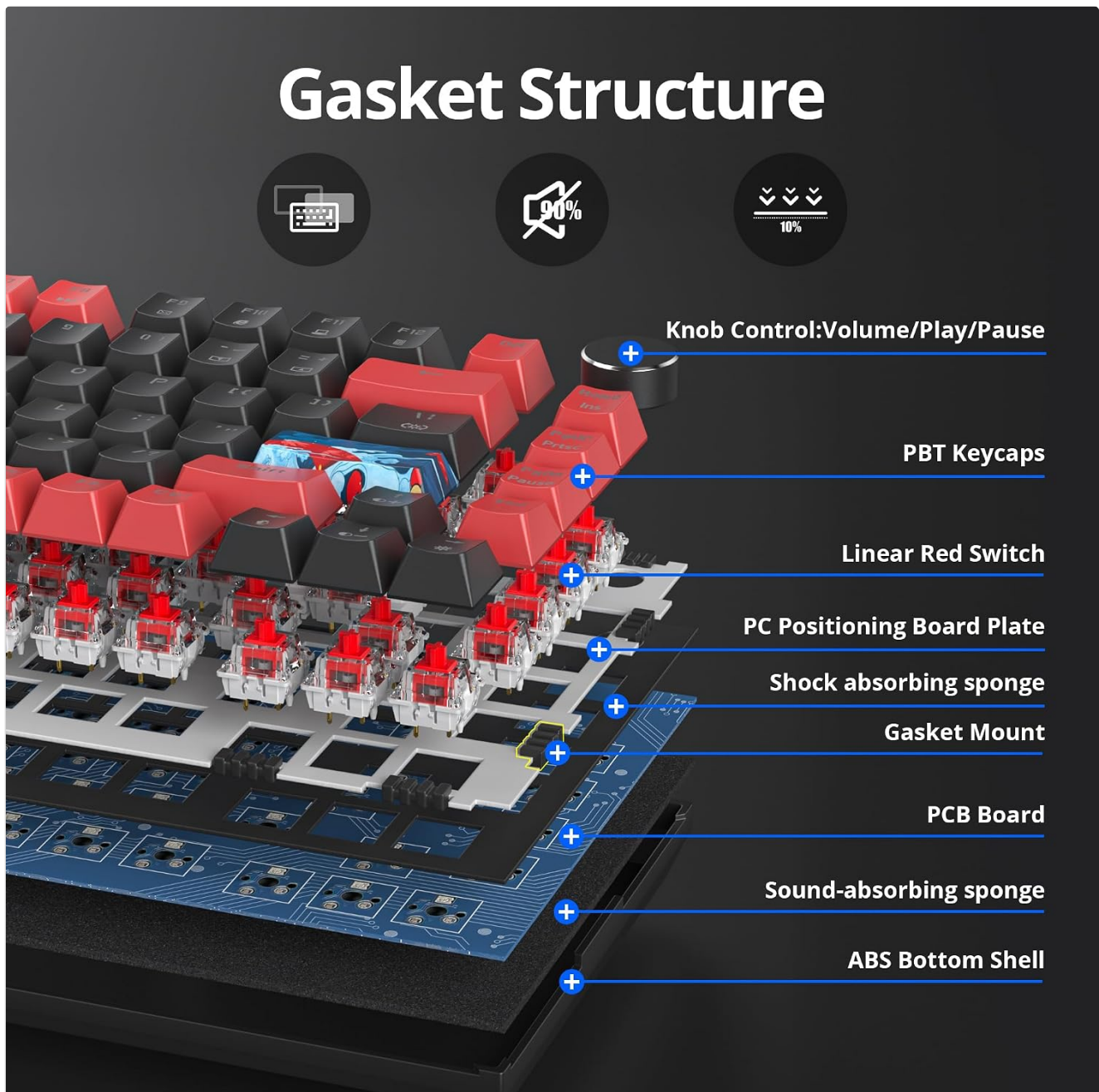
Image 3.1: Diagram illustrating the internal gasket mount structure, PBT keycaps, and linear red switches.
