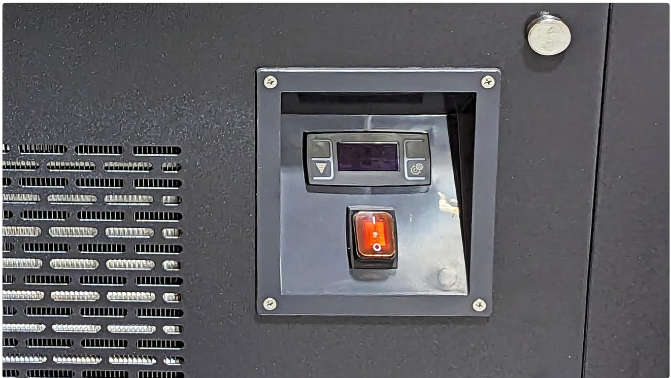
Figure 3: Digital temperature controller and power switch.
