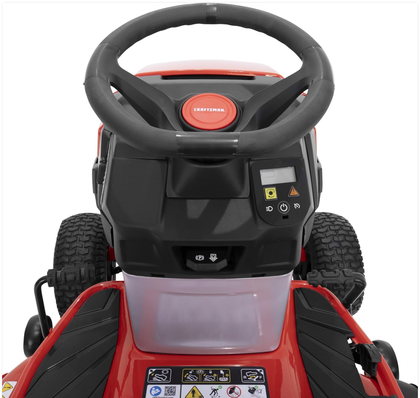
Figure 4.1: Detailed view of the Craftsman riding mower's dashboard, showing the steering wheel, display, and various control buttons including those for headlights and cruise control.
