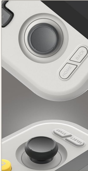
Figure 3: Overview of button layout, analog triggers, and 3D Hall Sticks.
