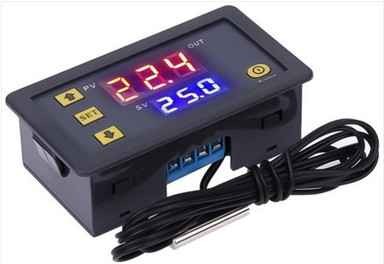
Figure 5.1: Wiring terminals and sensor connection on the W3230 controller.
