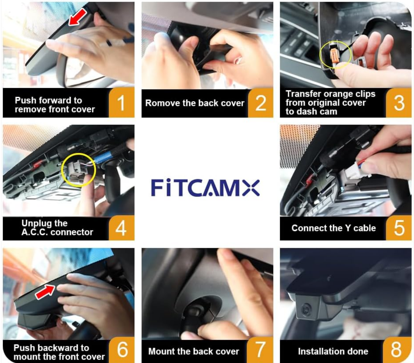
Figure 2: Visual guide detailing the 8 steps for installing the Fitcamx dash cam. This includes removing the front cover, transferring clips, connecting cables, and reassembling the unit.
