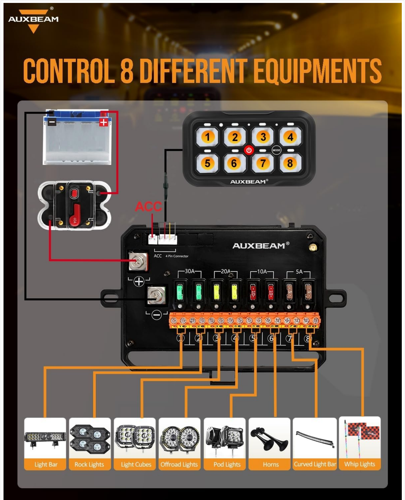
Figure 4: Detailed wiring diagram for connecting the switch panel to various accessories.
