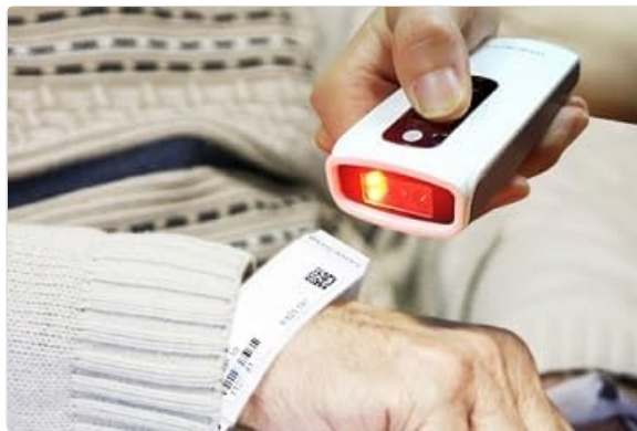
Figure 3: The MT850-USBC scanner in use, reading a barcode on a wristband. This demonstrates the scanner's application in medical or service environments, showing its red scanning light active.
