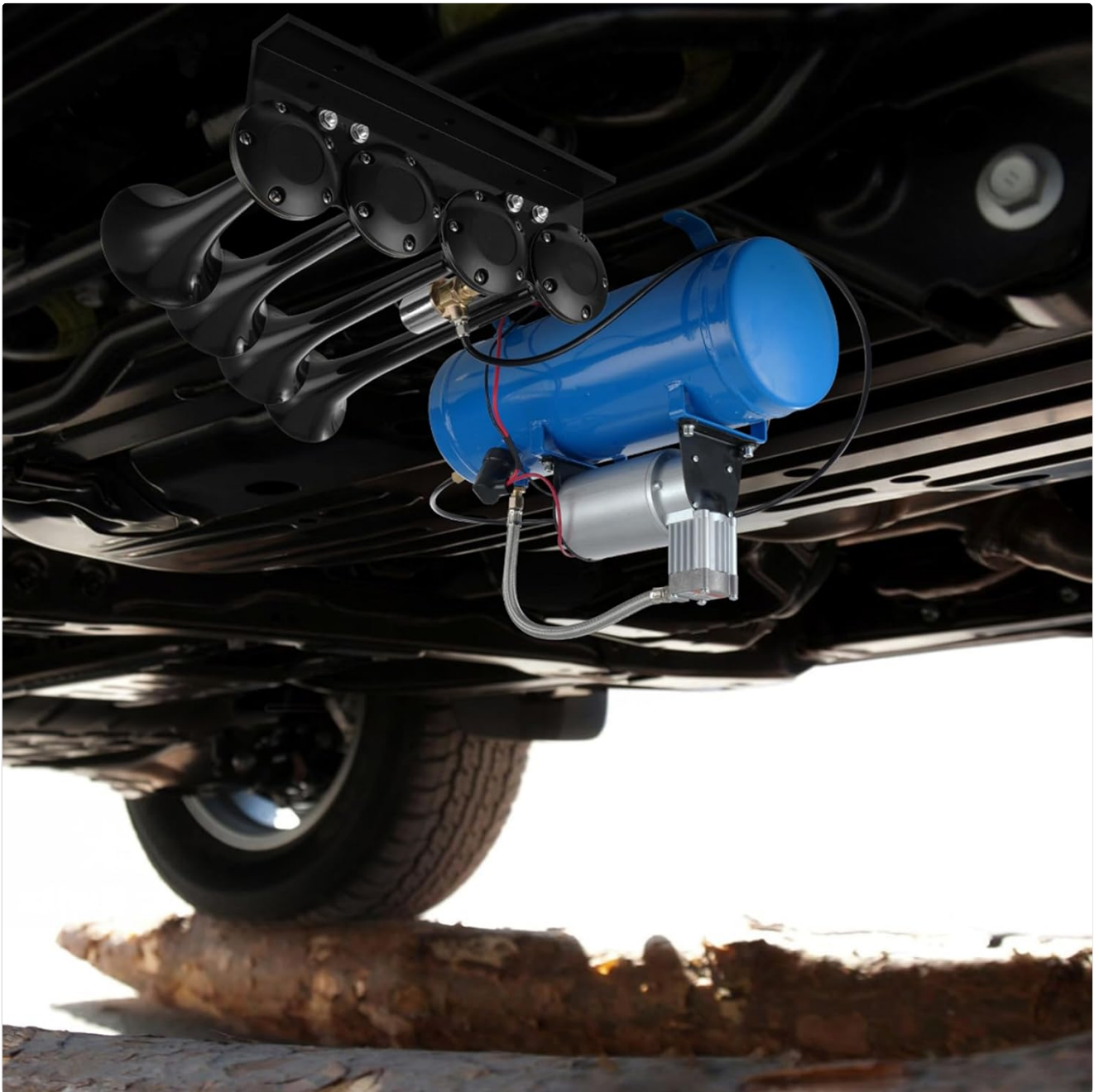
Image: An example of the horn kit installed underneath a vehicle, demonstrating a common mounting position for optimal performance and protection.
