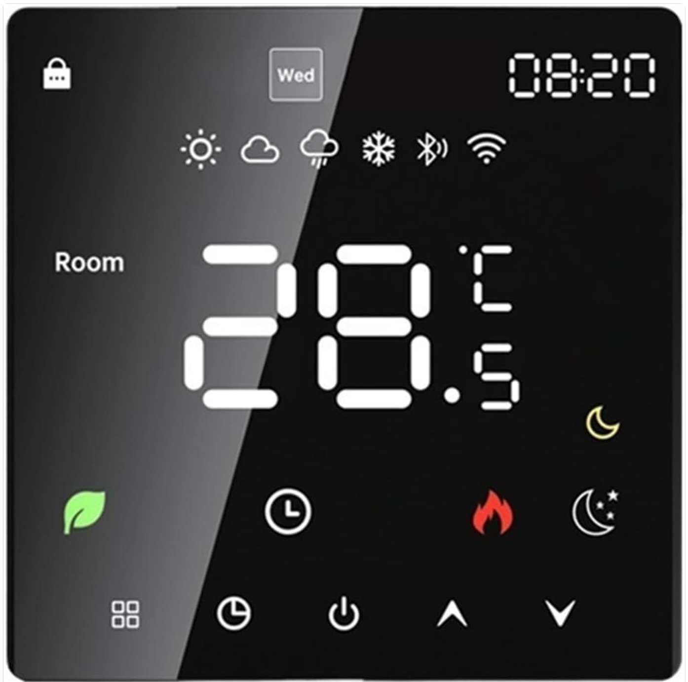
Figure 4.1: Front view of the CEMELI Smart Thermostat display, showing current temperature, time, and various status icons.
