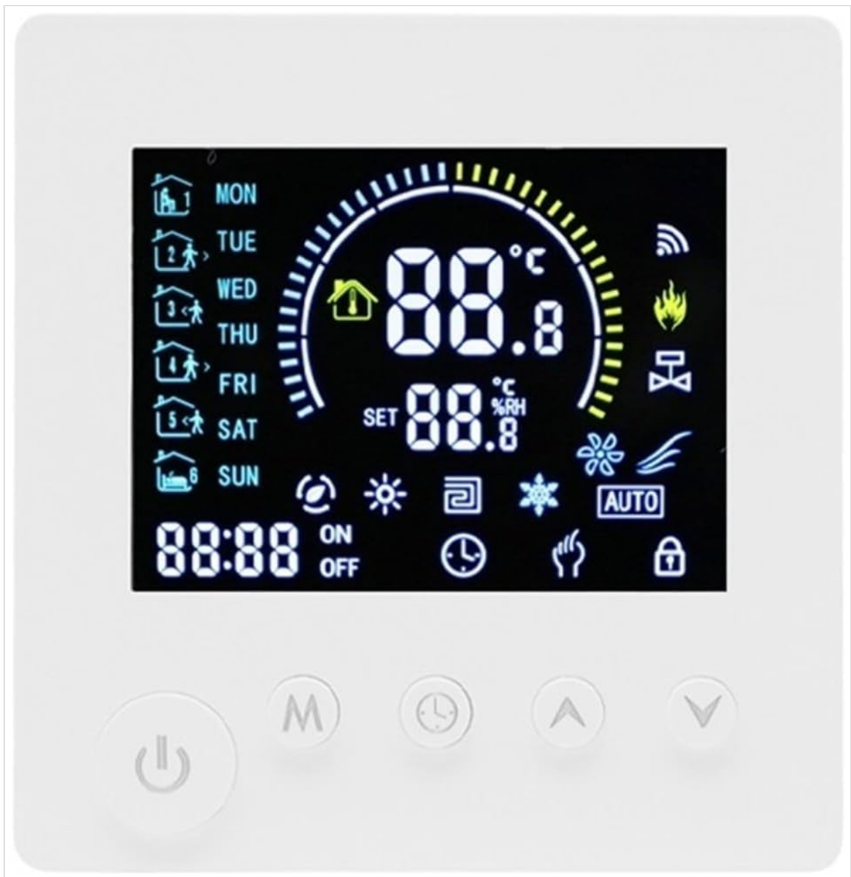
Image: Front view of the COKYIS WiFi Thermostat K1MRH3A. The LCD screen displays the current temperature (88.8°C), set temperature (88.8°C), day of the week (MON-SUN), time (88:88), and various status icons including WiFi signal, heating indicator, and auto mode. Below the screen are physical buttons for power, mode, clock, up, and down.
