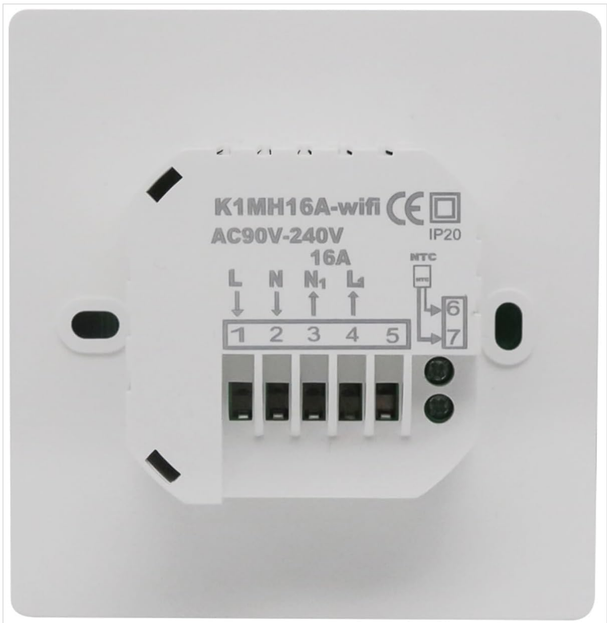
Image: Rear view of the COKYIS K1MH16A-wifi thermostat showing the wiring terminals. Terminals 1 and 2 are for the power supply (L and N), terminals 3 and 4 are for the heating load (N1 and L1), and terminals 6 and 7 are for the NTC temperature sensor. This diagram is crucial for correct electrical connection.
