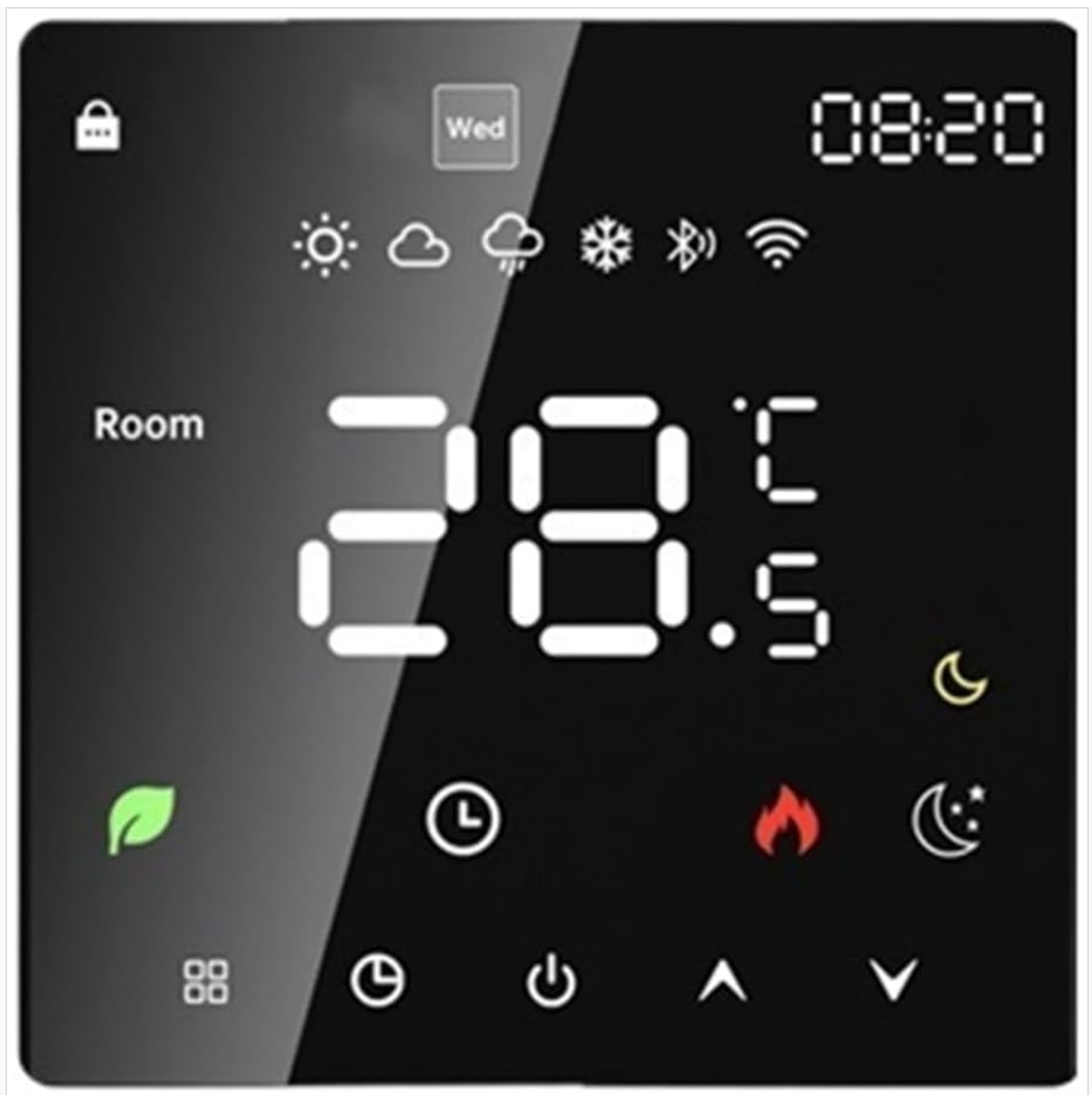
Figure 1: Front view of the CEMELI K6H-3A Smart Thermostat. The display shows the current room temperature, time, day of the week, and status icons for Wi-Fi, heating mode, and child lock. Touch buttons are located at the bottom for power, mode, and temperature adjustment.
